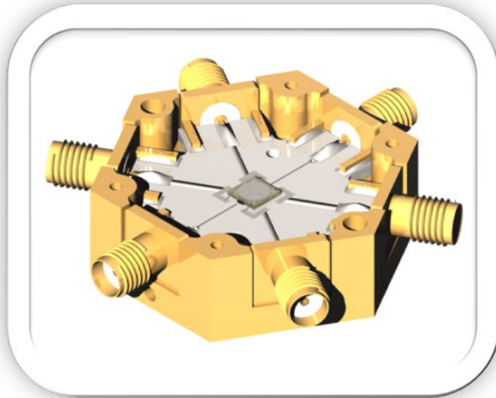
Figure 23: MSL-DD-04 is a quadrant diamond detector designed and made by Micron Semiconductor Ltd. The versatility of the board and casing designs allows for the accommodation of CVD diamonds of different sizes and thicknesses.
