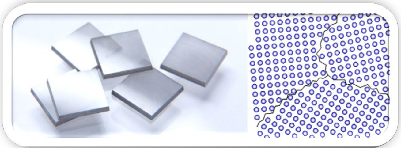
Figure 13: Left – At the macro scale and under natural light single crystal and polycrystalline diamonds are indistinguishable (courtesy of Element6).
